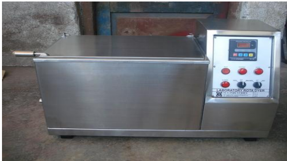
Fig 3. Sample dyeing Machine
